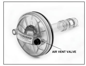
...THROUGH THE PUMP UNION RELEASING AN AIR LOCK ...
